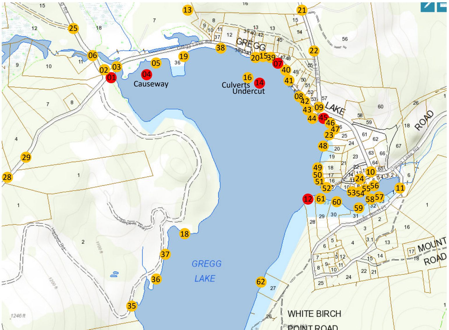
Figure 3.1. Erosion “hotspots” identified in the Gregg Lake watershed in the vicinity of the northern part of the lake. Locations classified as “high impact” (red dots) were estimated to cause phosphorus loading in the range of 1.5–2.5 lb/yr, whereas “medium impact” sites (orange dots) were estimated to supply 0.1–1.5 lb/yr. Sites 1–31 were evaluated by FBE for pollutant loads; sites 32–63 were rated by comparison with FBE’s assignments.
